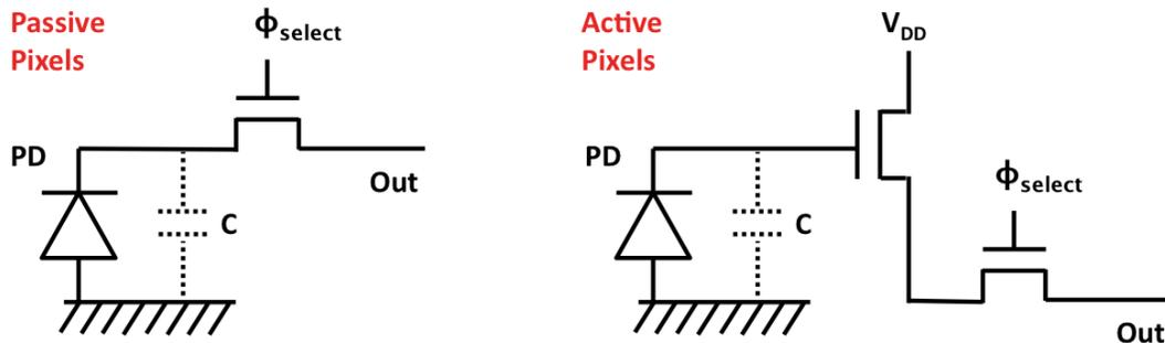
Figure 1.5: A simplified diagram that shows the main difference between the passive and active pixel CMOS architectures. In the passive version, the charge in the pixel is fed through the column bus directly to the output. In the active version, a source follower MOSFET buffers the voltage stored on the capacitance of the pixel.
