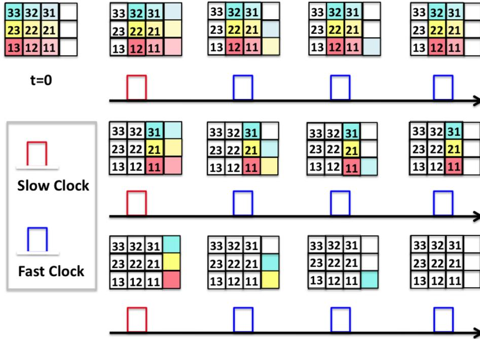
Figure 1.3: A simple cartoon showing the process of clocking in a CCD. The numbers of the pixels designate their physical location in the CCD. The colors have no relationship to wavelength or color of photons; they are solely meant to keep track of charge packets. Only one clock is shown for each fast and slow cycle in this illustration. Time moves from left to right and then down.
