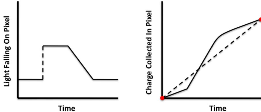
Figure 1.4: A simple cartoon showing a transient astronomical event such as a flaring M star and how the CCD perceives it. The left figure shows the number of photons hitting the pixel vs. time. The right figure shows the charge collected in the pixel as a function of time. The only data points available to the observer are the red dots, leaving the actual light curve of the object a mystery.
