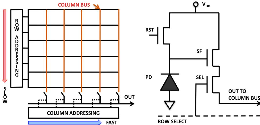
Figure 1.6: (Left) Diagram of a simple 5x5 CMOS multiplexer with one output, following Magnan [17]. The slow and fast read directions are indicated by the colored arrows and the column buses are indicated as the orange lines. (Right) 3T pixel schematic showing the reset transistor (RST), source follower transistor (SF), row select transistor (SEL), photodiode (PD), and the supply voltage  $V_{DD}$ .
