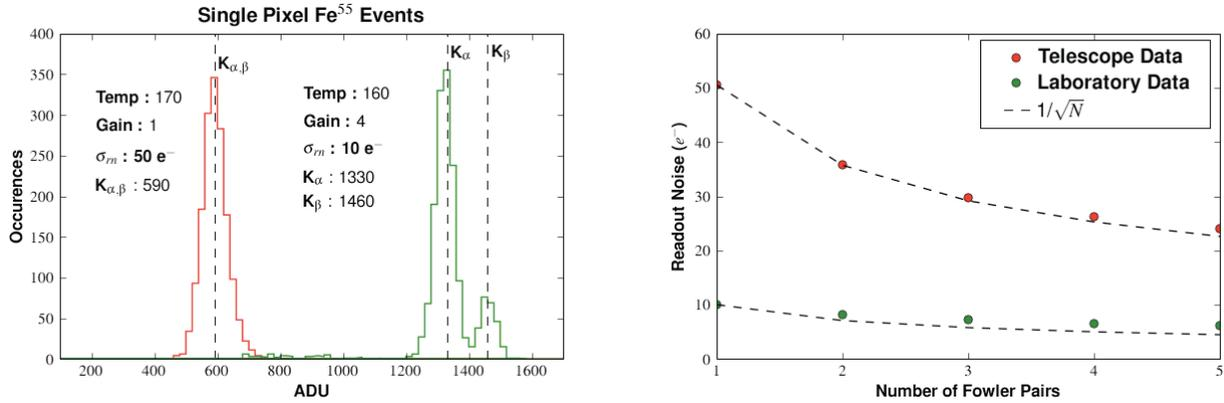
Figure 7. **Left)** Comparison of Fe<sup>55</sup> histograms from data taken while at telescope (left histogram) and in laboratory after noise reduction (right histogram). The separate peaks are clearly visible in the laboratory data, indicating noise improvement and diminished crosstalk. **Right)** Comparison of read noise from data taken while at telescope (top curve) and laboratory data (bottom curve). The temperatures and gains for the two curves are the same as the ones in the left plot.
