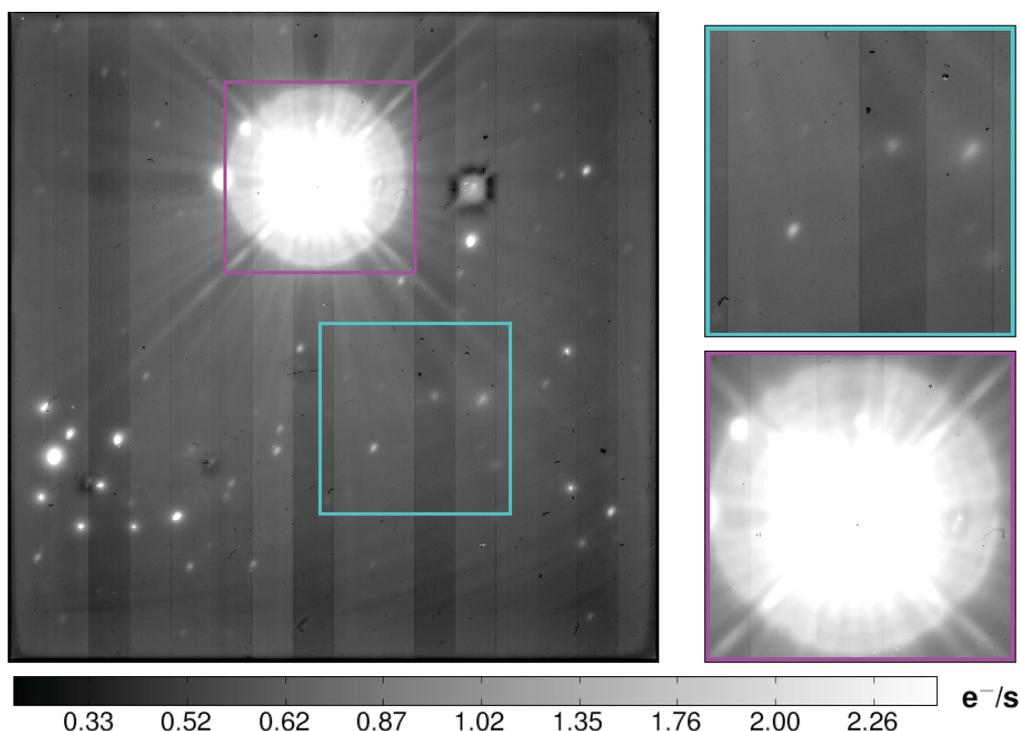
Figure 3. (Left) Full frame slopefit to a 1770 s exposure taken with H1RG-022 with no guiding. (Right) A zoomed view of the box enclosing the very saturated star SAO 54817 is shown at bottom right. The light from this star has consumed a circular region of pixels with a radius of 50 pixels. The box at upper right shows an area away from the guide window that contains three stars of irregular shape. Both boxes are  $300 \times 300$  pixels.
