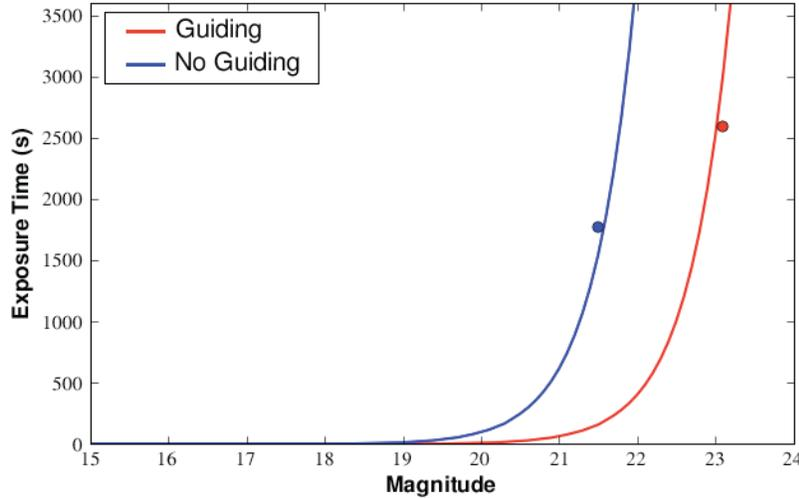
Figure 6. Theoretical exposure time required to reach limiting magnitude with a signal to noise ratio of 3 for the cases where the telescope is being guided by H2RG-32-147 (right curve) and where it is simply trying to track stars at the sidereal rate with H1RG-022 (left curve). The data points are also plotted as circles. The difference is due almost entirely to the disparity in point spread functions.
